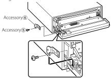
4 Tighten the screw (ø2 × 5 mm) (Accessory (5)) and bracket (Accessory(7)) in the hole shown on the diagram.
